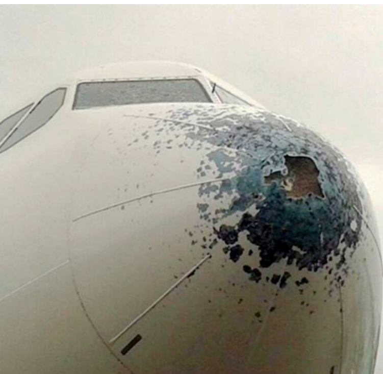
An aircraft radome damaged by hail storm. (credit: Ricardo Cirrielli)
