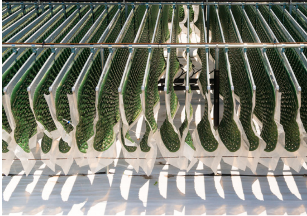
Rows of photobioreactors containing blue-green algae hang in the sun. CO 2 is captured from the air and pumped into the photobioreactors, where the cyanobacteria use sunlight to convert the carbon dioxide to fuel.
